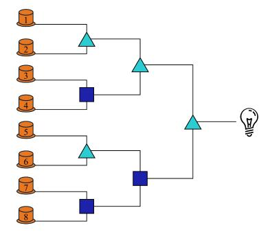
A triangle box will send on a signal if it receives signals from *both* incoming wires.
