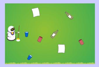
The robot starts by identifying the closest item. The robot then moves to this item and picks it up. Then the robot identifies the remaining item that was closest to the item it just picked up, and moves to this new item. The robot continues this process until all of the items have been picked up.
