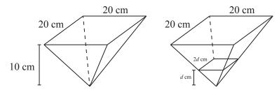
This is because, as Tank D fills, the ratio of the side length of the base to the height will remain constant. This ratio for the whole tank is 20 cm : 10 cm which is equivalent to 2:1. We could say that the square-based pyramid formed by the water at any instant is similar to the Tank itself.
